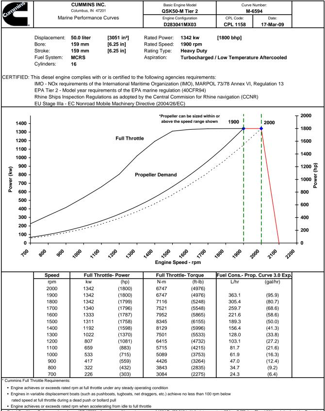
Rated Conditions: Ratings are based upon ISO 15550 reference conditions; air pressure of 100 kPa [29.612 in Hg], air temperature 25deg. C [77 deg. F] and 30% relative humidy. Power is in accordance with IMCI procedure. Member NMMA. Unless otherwise specified, all data is at rated power conditions and can vary ± 5%.
